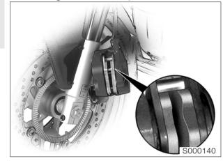
• Check/measure thickness of brake pads.
