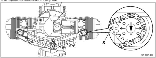
• Lock engine at firing TDC by inserting pin, **BMW No. 11 2 650**, through holes in clutch housing and engine block.
