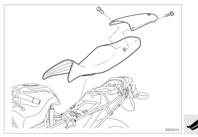
Removing and installing seat
