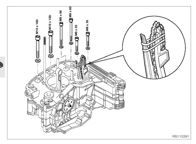
• Bolt the crankcase sections together.
