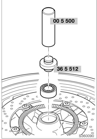
• First insert wide bearing using drift, BMW No. 36 5 512, and handle, BMW No. 00 5 500.
