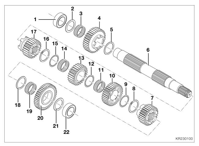
Disassembling/assembling output shaft
