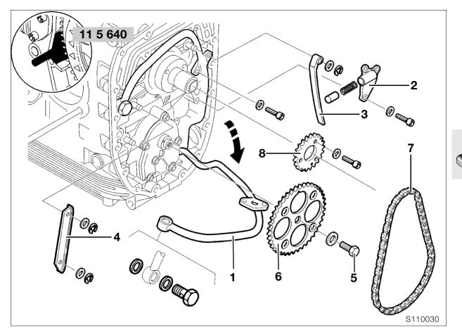
Removing auxiliary shaft drive
