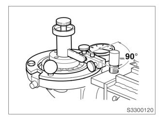
• Using the balls of your hands, press the crown wheel into the housing and turn it to and fro to check tooth backlash.
