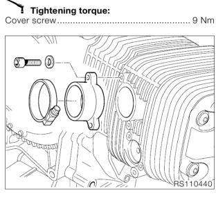
• Secure air intake stub pipe.
