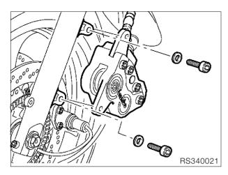
• Remove brake caliper.
