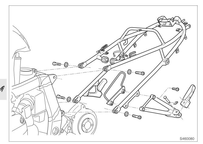
Removing and installing frame tail section
