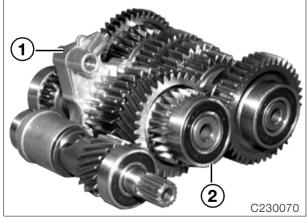
• Insert selector fork (1) into intermediate shaft (2).
