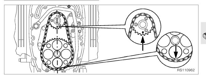
Left cylinder = at firing TDC: marks (arrows) on chain sprocket/auxiliary shaft and chainwheel/crankshaft at bottom
