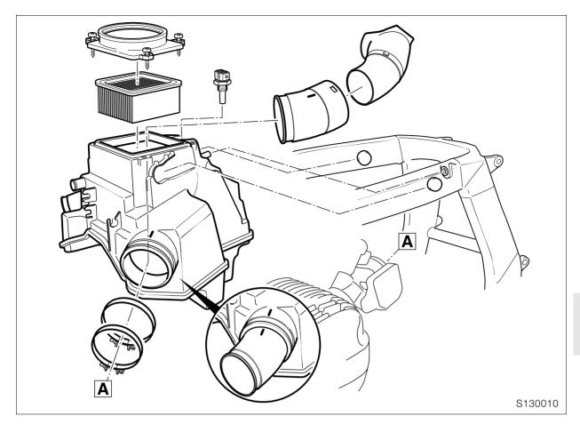
Removing and installing air filter housing
