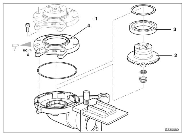
Removing and disassembling crown wheel
