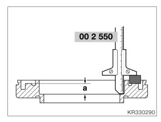
• Using depth gauge, **BMW No. 00 2 550**, measure distance a.
