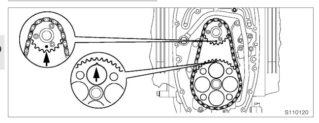
Right cylinder = at firing TDC: marks (arrows) on chainwheel/auxiliary shaft and chain sprocket/crankshaft are aligned.
