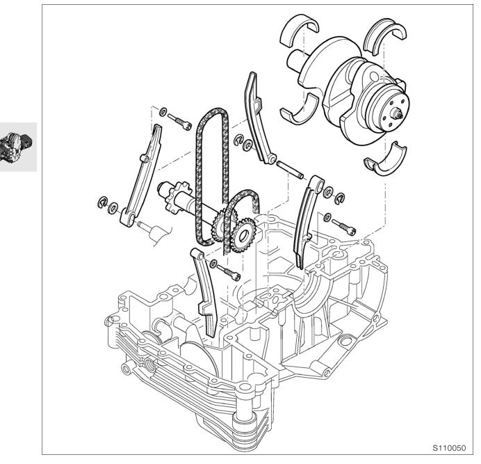
Removing crankshaft, auxiliary shaft and timing chain tensioning and slide rails
