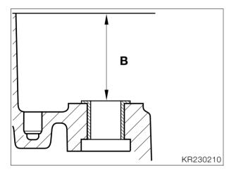
• Measure dimension **"B"** from shouldered bushing to housing mating face.
