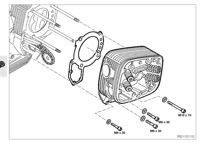
Removing cylinder head
