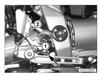
• Insert a feeler gauge of the correct thickness between the adjusting screw/brake lever and the stop (arrow).
