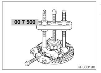
• Using puller, **BMW No. 00 7 500**, pull taper roller bearing off crown wheel.
