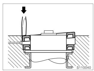
• Carefully lever out radial shaft seal, using a screwdriver.
