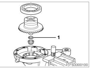
• Compensate for excessive backlash by inserting a thinner shim washer, and for insufficient backlash by inserting a thicker shim washer (1).
