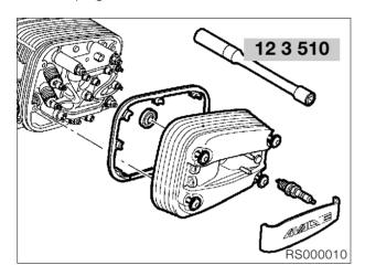
Install spark plugs with spark plug socket wrench, **BMW No. 12 3 510**. •
