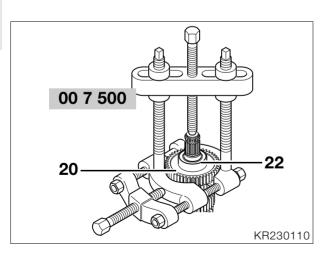
• Using universal puller, **BMW No. 00 7 500**, pull off grooved ball bearing (22) together with 1st gear wheel (20).
