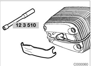
• Remove spark plugs with the spark plug wrench, **BMW No. 12 3 510**.
