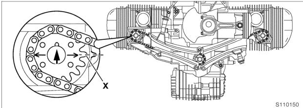
Lock engine at firing TDC by inserting pin, BMW No. 11 2 650, through holes in clutch housing and engine block.
