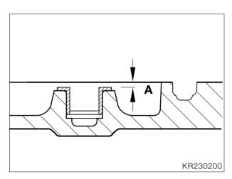
• Measure dimension **"A"** from shouldered bushing to cover mating face.
