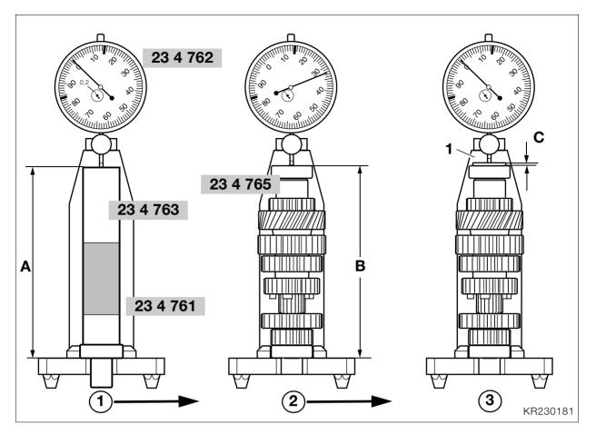
Checking/adjusting fully assembled length of gearbox shafts and selector drum
