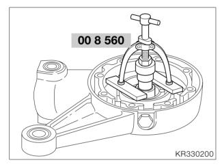
• Pull out the outer race using internal puller, **BMW No. 00 8 560**.
