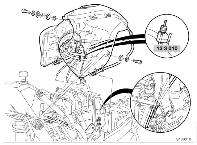
Removing and installing fuel tank
