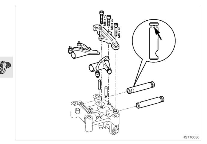
Disassembling/assembling valve gear holder
