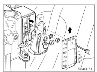
[ABS] Remove cover and disconnect cables.
