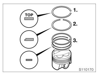
Carefully fit piston rings to piston in the following sequence, using piston ring pliers: 3rd groove - 3-S ring
