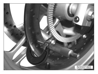
• Examine the brake discs carefully for cracks, damage, distortion, wear and score-marks.
