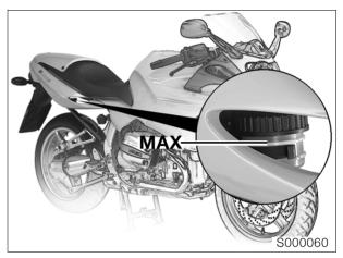
• Check the brake fluid level by looking through the opening in the right-hand side panel.
