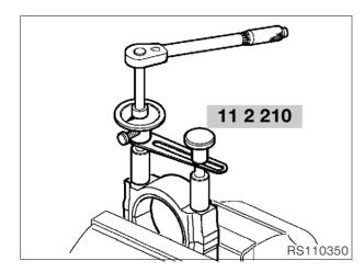
Install bearing shells and assemble conrods.
