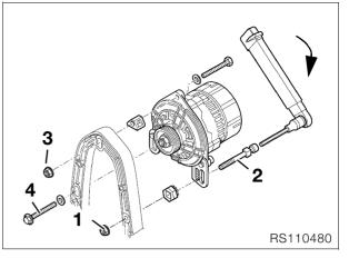
Slacken alternator mounting screws and nuts (1,3,4) and install a new Poly-V belt if necessary.
