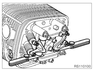
• Adjust the holder for minimum end float.
