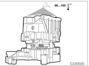
• Heat the bearing seats in the housing to 80 ... 100 °C (176...212 °F) and place the housing on the cover.
