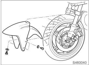
• The front wheel has to be removed to permit re-moval of the front mudguard.
