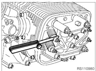
• Check valve clearance with feeler gauge and, if necessary, correct with adjusting screw.
