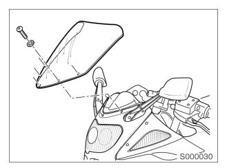
• Carefully tighten the securing screws by hand.
