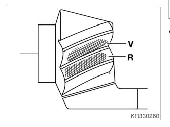
• If the correct shim is installed, the following contact pattern appears with no load applied.
