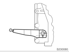
Install shift lever in correct position. •
