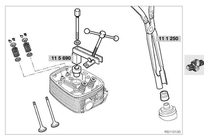
Disassembling, checking, repairing and reassembling cylinder head
