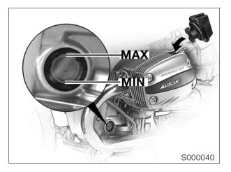
Check the oil level with the motorcycle upright: if necessary, use stand, **BMW No. 00 1 560**, to keep the motorcycle in the upright position.
